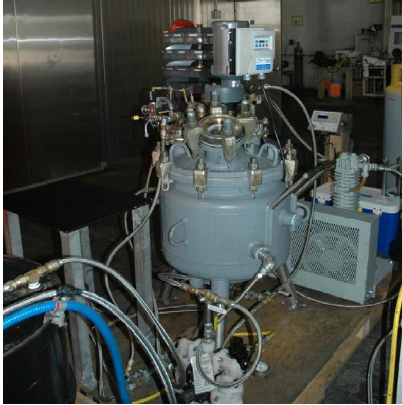
Figure 10. HFC-227ea/SBC HHFE filling station.
