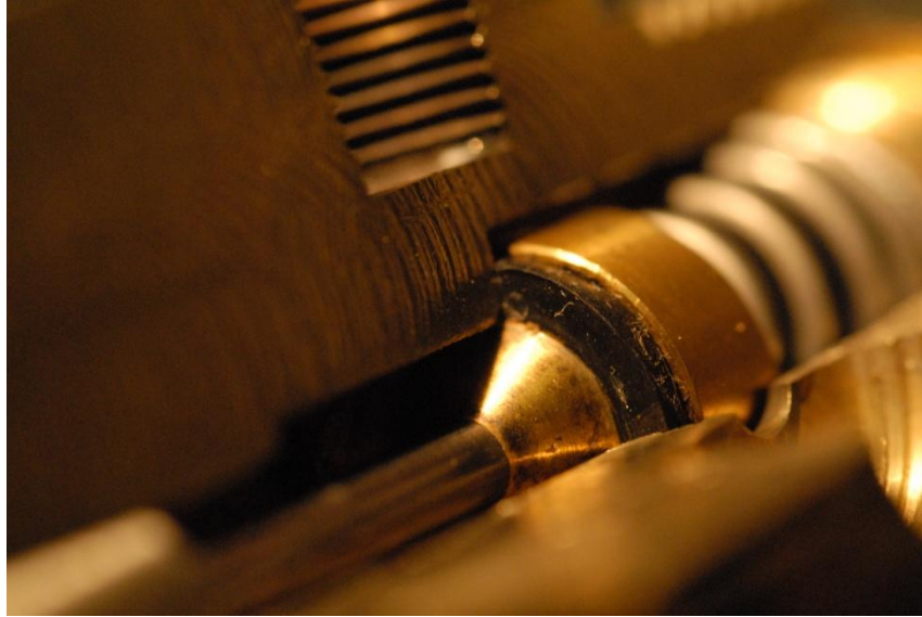
Figure 12. Photograph of the valve seat cut to show internal surfaces.
