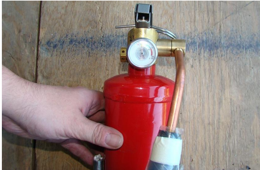
Figure 14. Photograph of damaged handle and pull pin after a drop test.
