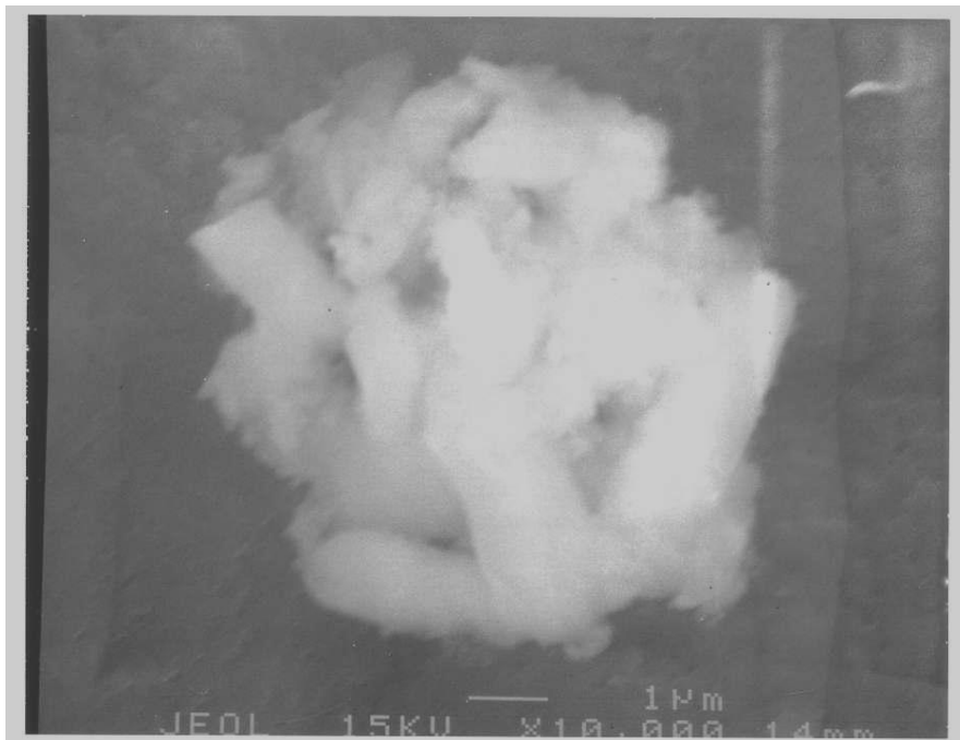
Figure 8. FESEM showing morphology of Quickfire USA SBC powder
