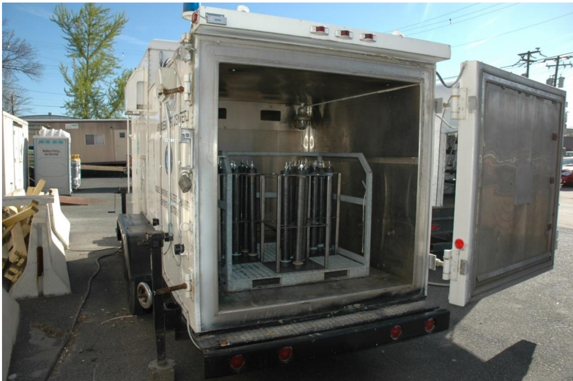
Figure 30. Thermal cycling chamber with rack containing accelerated aging (diurnal) samples.
