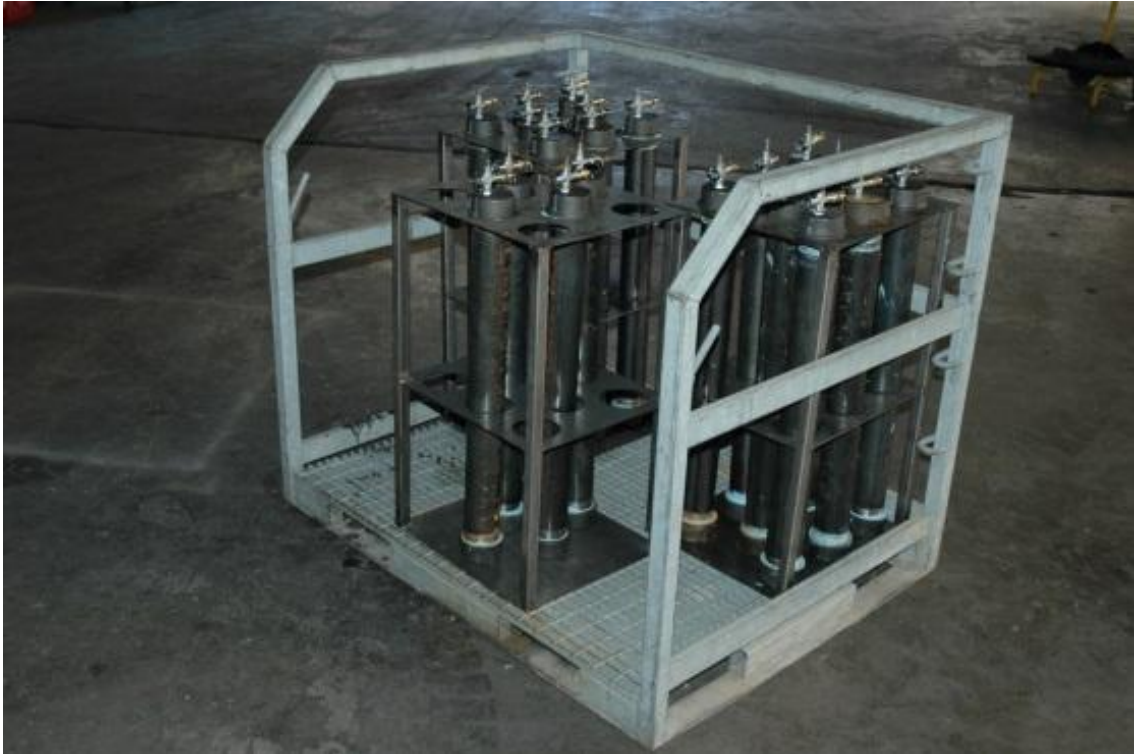
Figure 29. Overpressure tubes in vertical tube holder mounted on mobile rack.
