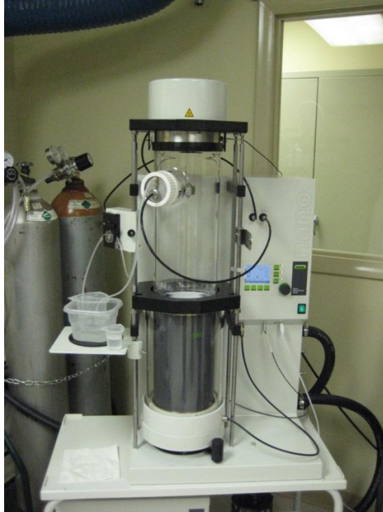
Figure 20. Buchi – B90 bench scale spray dryer used in test of various process flow and heating conditions
