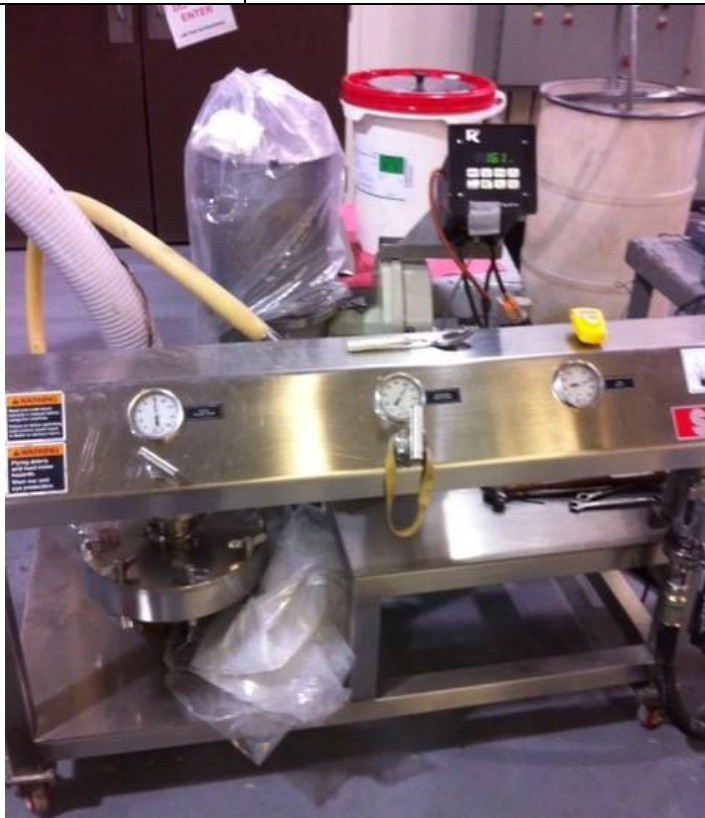
FIGURE B-1. Photograph of jet-milling equipment.
