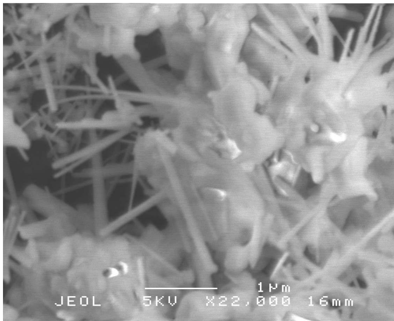
Figure 20. Buchi B90 Powder FESEM (Spray Drying of SBC Solution)
