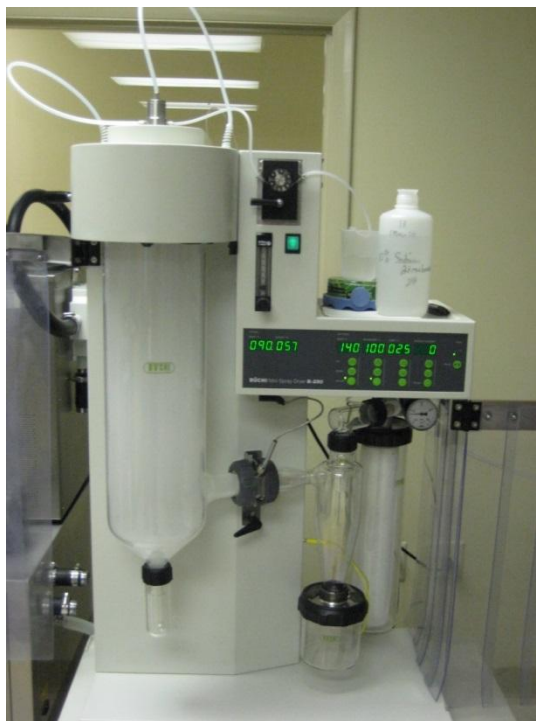
Figure 18. Buchi – B290 bench scale spray dryer used in test of various process flow and heating conditions
