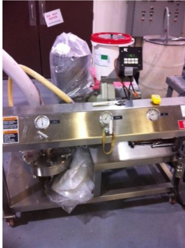
Figure 16. Jet-mill used in production of SBC.
