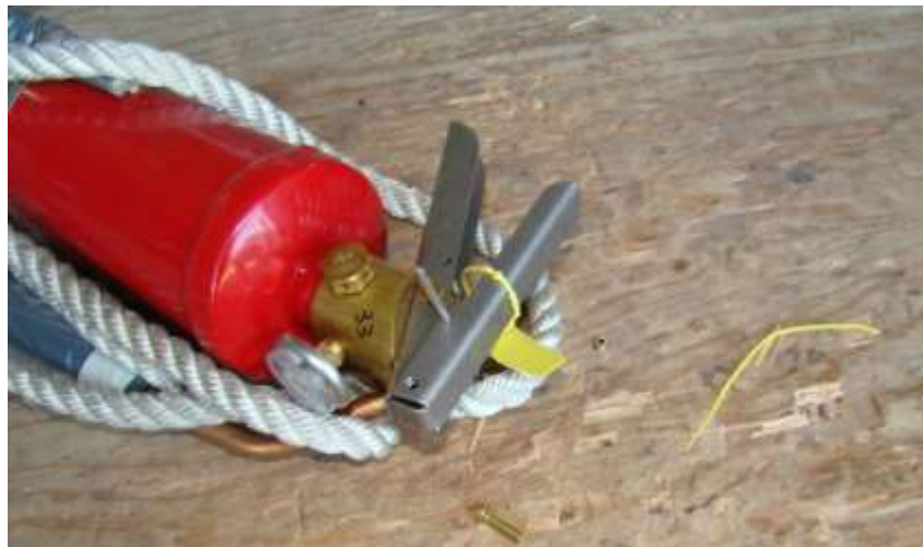
Early Drop Test sample that resulted in a bent pull pin, rivet and handle
