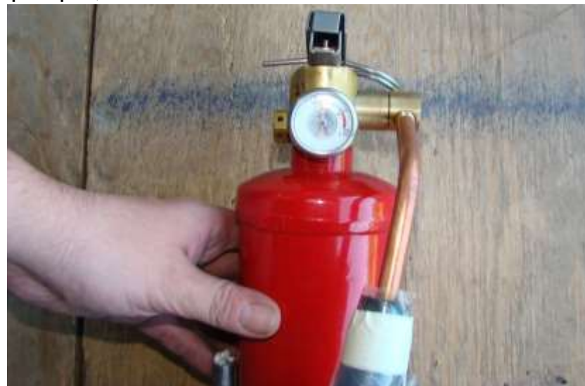
Early Drop Test sample that resulted in a bent pull pin, rivet and handle
