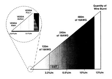
Figure 1: Smoke Obscuration measured based on a Burning wire within a 1000m<sup>2</sup> room
