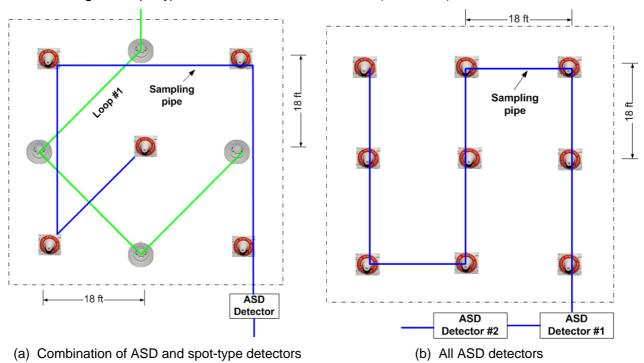
Figure 6: ASD for double knock (coincidence) detection scheme
