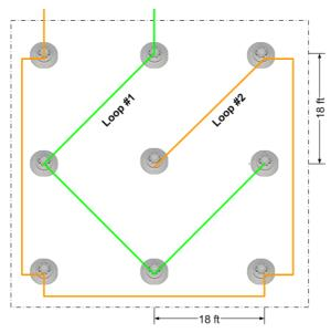
Figure 5: Spot-type detectors as standard double knock (coincidence) detection scheme
