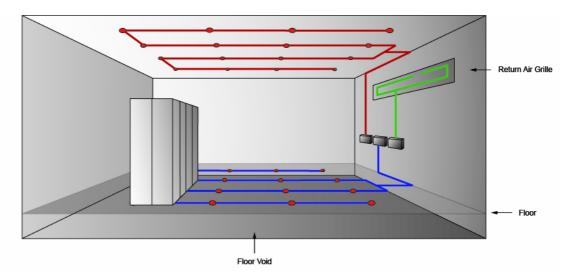
For ASD detector, average transport time was used. For spot-type detectors, the detector activation relies on number of factors including temperature raise, air velocity and smoke density [17]. To simplify the analysis, 20 seconds entry lag time were adopted as a conservative approximation to the spot-type detectors after the smoke density has reached the detector nominal sensitivity.
