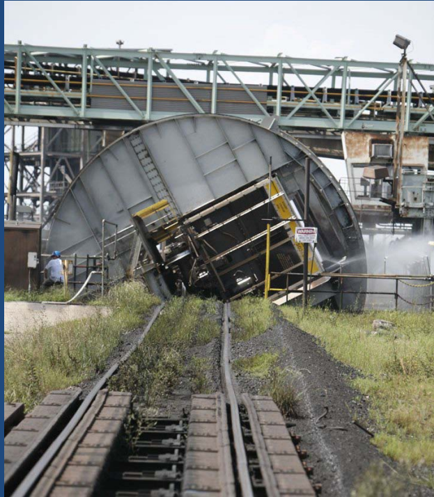
Rail car (rotary) unloader
