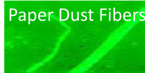
Soft Tissue Papermachine Dust -400X
