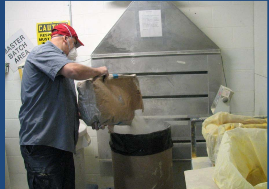
Bag unloading stations
