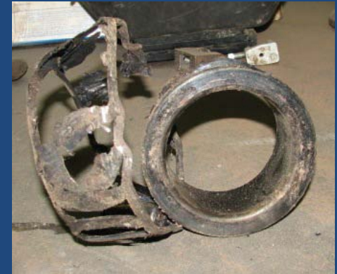
Failed bearing ignition source for feed plant dust explosion
