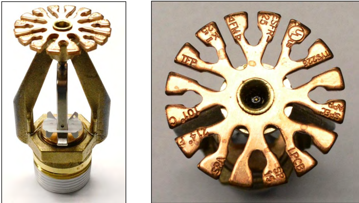
Figure 2 Test Sprinkler Photos
