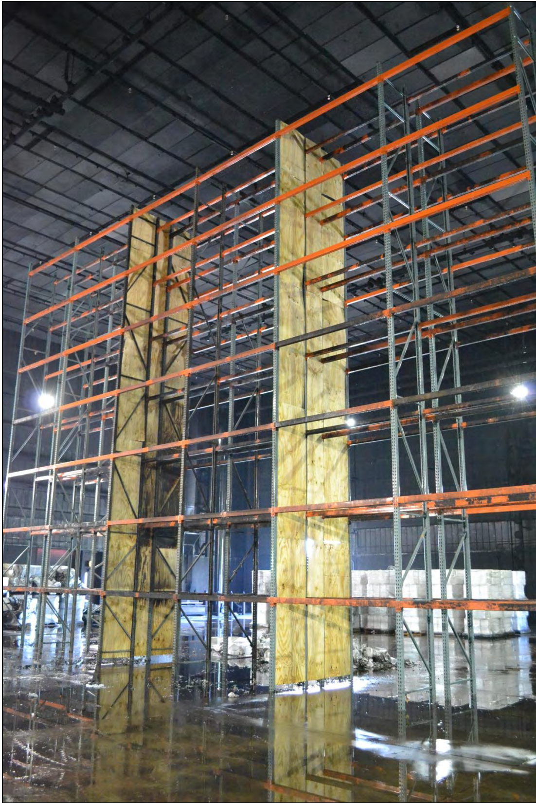
Figure B- 7 View of Combustible Barriers from the Southeast with Commodity Removed
