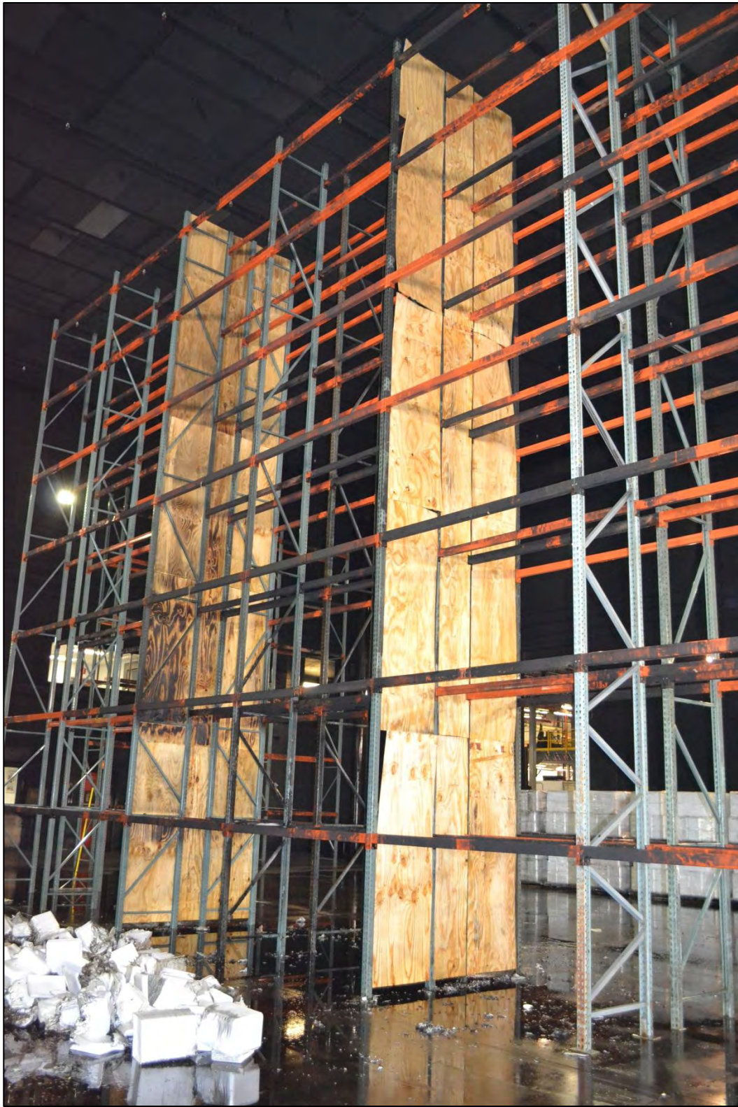
Figure B- 8 View of Combustible Barriers from the Southeast with Commodity Removed
