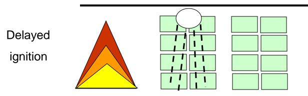
Liquid spray from bursting aerosols rains out affecting lower levels
