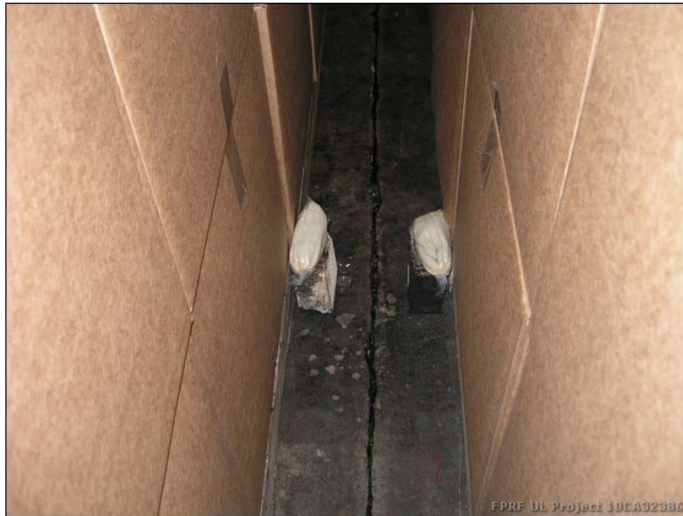
Figure 28 Test 4 Ignition Detail
