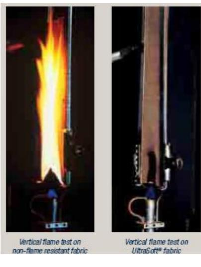
7.6 cm wide x 30.5 cm high (3 in. x 12 in.) rectangle samples tested before and after 100 cycles of washing and drying
