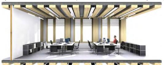
Figure 56 – Concrete floor slab over heavy timber beams (Wurm, Gockel, & Unger, 2012)
