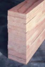
Figure 19 – Glulam beam (APA, Glulam Product Guide, 2008)
