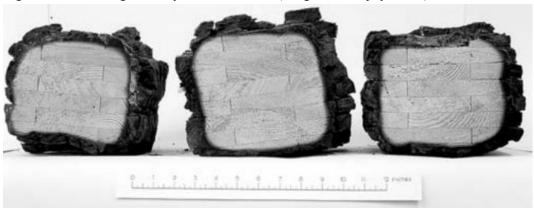
Figure 54 – Charring in heavy timber sections (Bregulla & Enjily, 2004)
