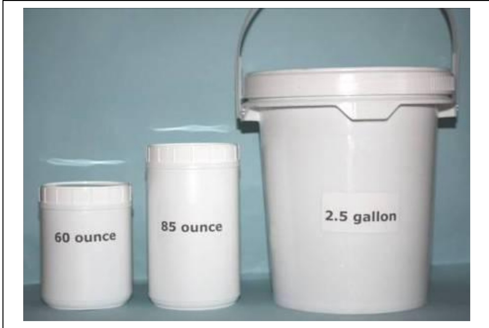
FIGURE 3. HDPE containers and pail used as combustible test packaging in intermediate-scale fire exposure tests. The 60 ounce HDPE container was used in a majority of the tests.
