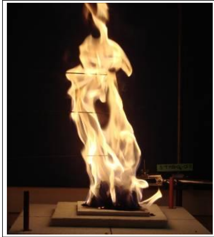
FIGURE 32. Photograph during screening test with 30 g, 3:7 potassium bromate:cellulose powder.
