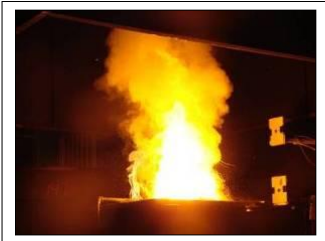
FIGURE 13. Photograph during fire exposure test with a packaged oxidizer.
