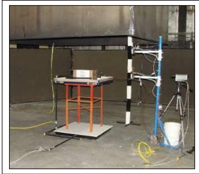
FIGURE 12. Photograph of the intermediate-scale fire exposure test set up under a 2MW hood.
