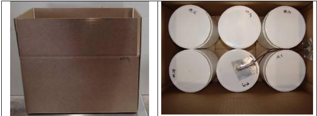
FIGURE 4. Combustible test packaging consisting of a doubled-wall carton (left) and containing six 60-ounce HDPE containers(right), each of which contained 4 pounds of granular, crystalline, or tablet form common salt or oxidizer.
