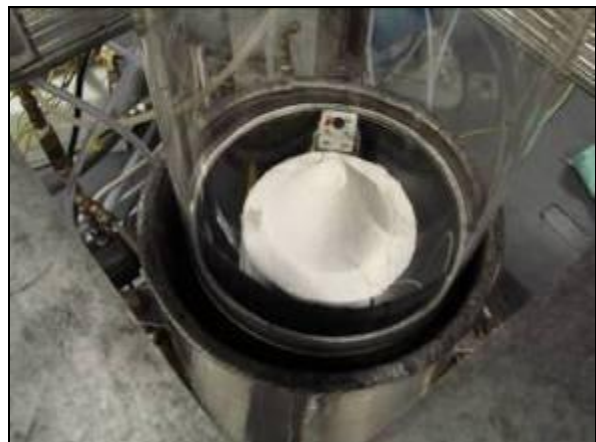
FIGURE 10. Photographs showing modified combustion-type test set up before and after addition of 30g pile of oxidizer-cellulose powder.
