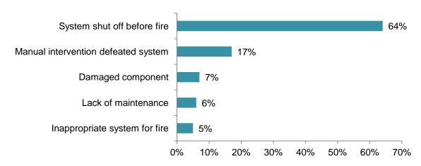
In 2007-2011 fires where sprinklers operated, they were effective in 96% of the cases. The graph below is based on the other 4% in which the sprinkler was ineffective.
