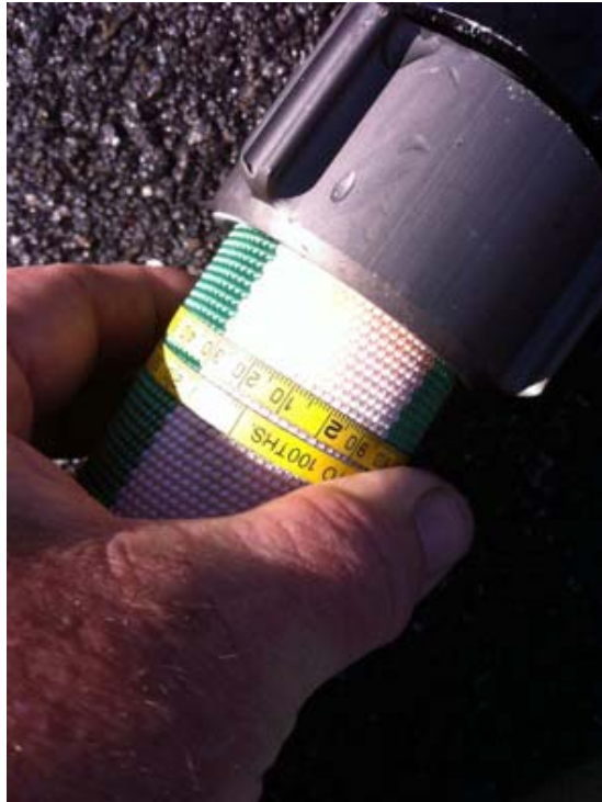
Figure2. Measurement of hose OD using a “plumbing tape” (MSEX)
