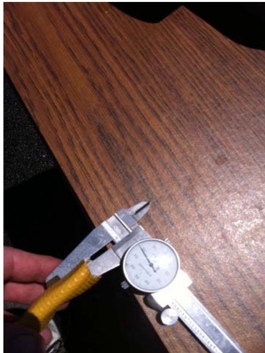
Figure3. Measurement of hose wall thickness (MSEX)
