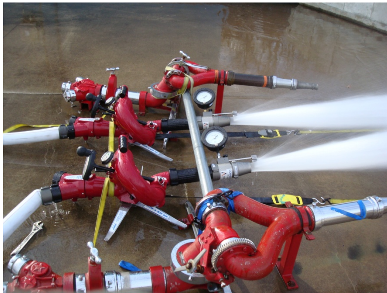
Figure 6. Multiple nozzle flow test at CONN
