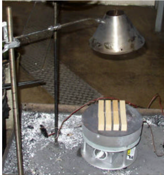
Figure 30 – Photograph of test set-up for UL 217 smoldering test
