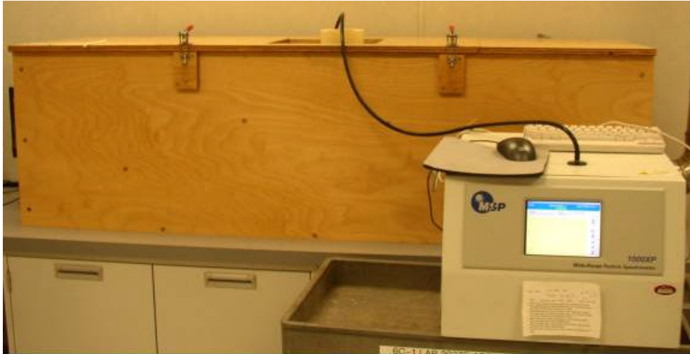
Figure 3 – WPS Spectrometer connected to the UL 217 Smoke Box
