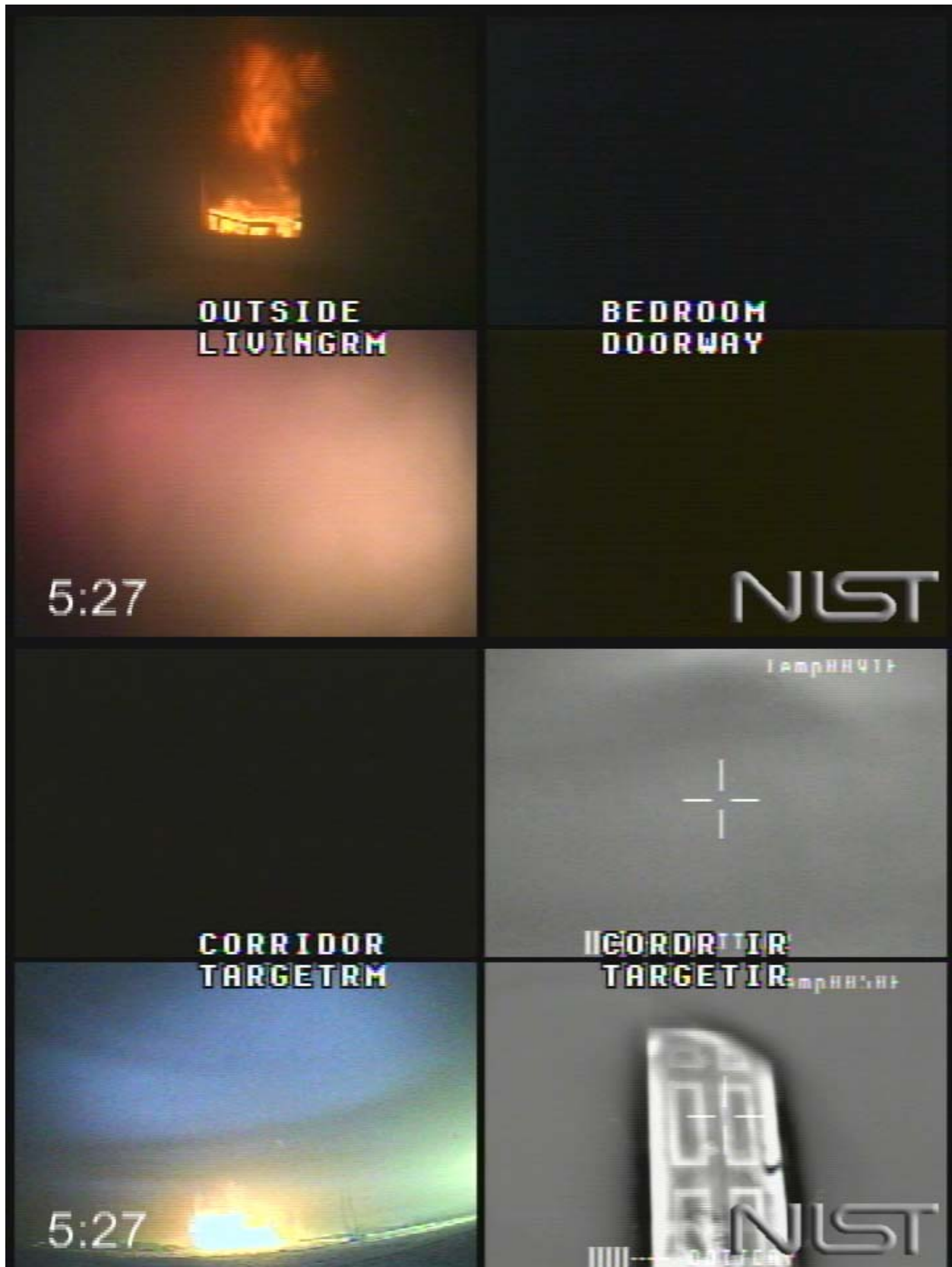
Figure 5.5.1-8. Experiment 5, WCD deployed, 327 s after ignition.
