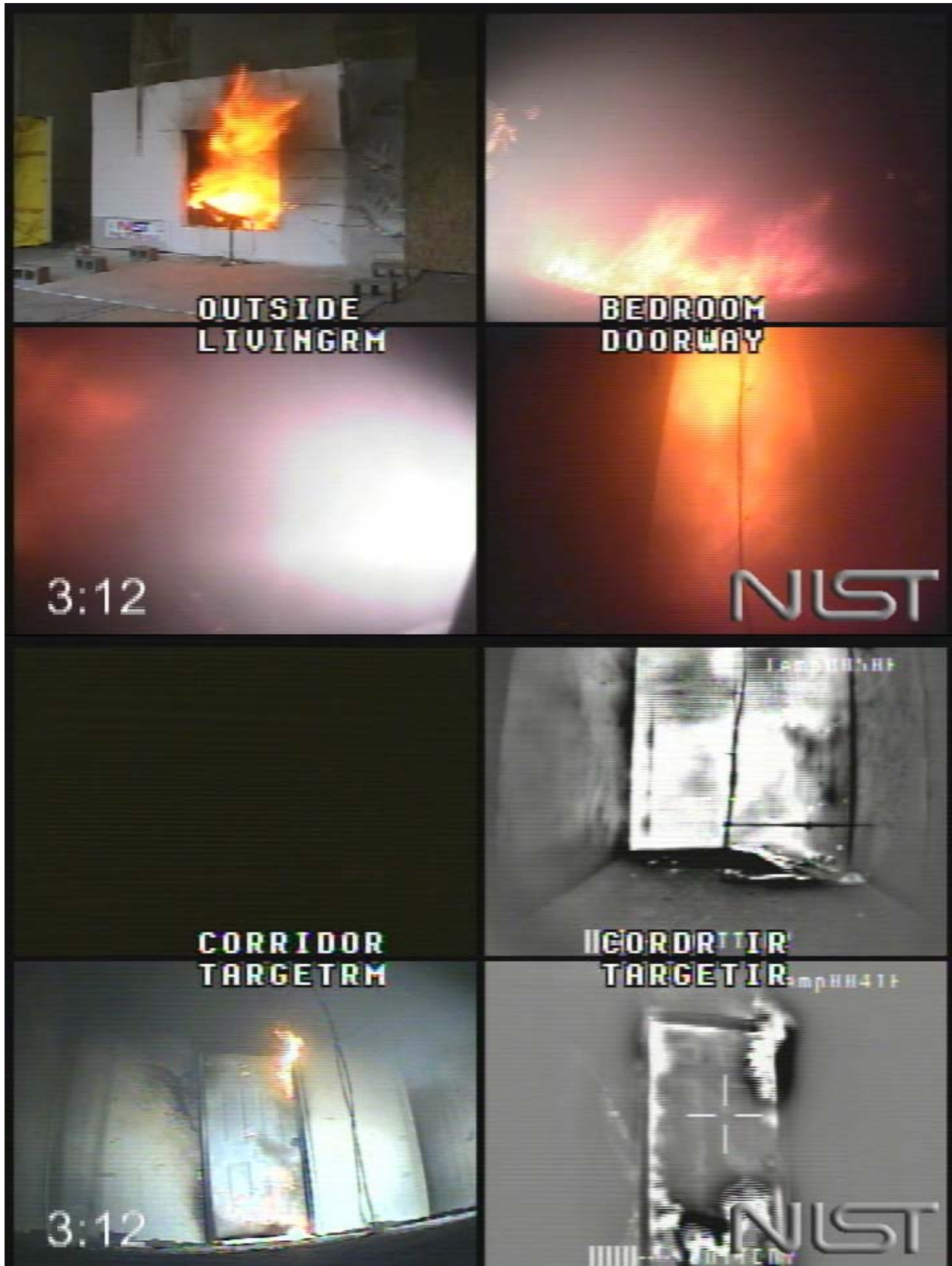
Figure 5.6.1-6. Experiment 6, corridor flames, 192 s after ignition.
