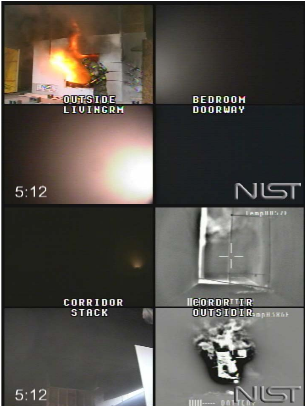
Figure 5.7.1-7. Experiment 7, window fully vented, 312 s after ignition.
