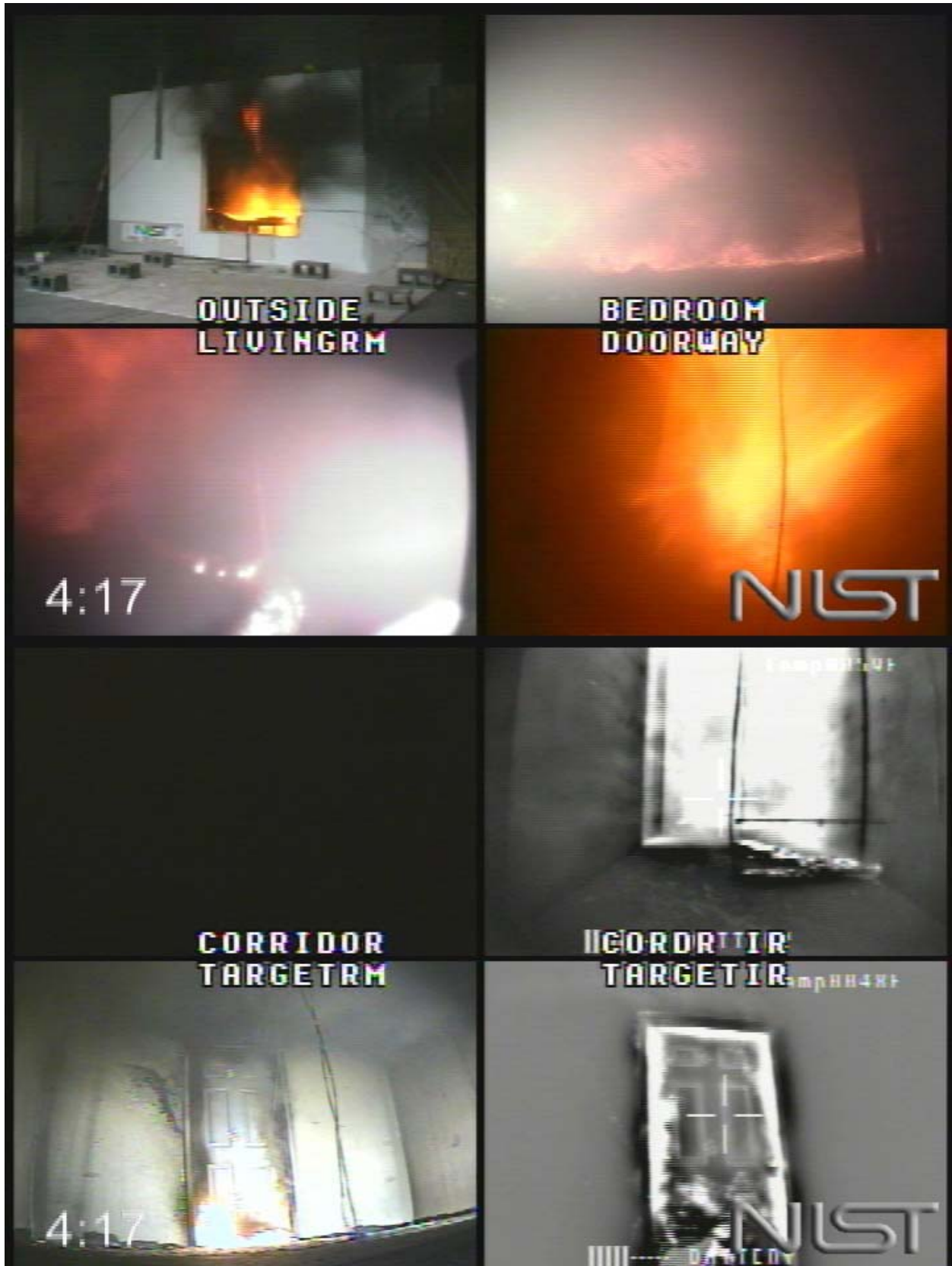
Figure 5.5.1-6. Experiment 5, corridor flames, 257 s after ignition.
