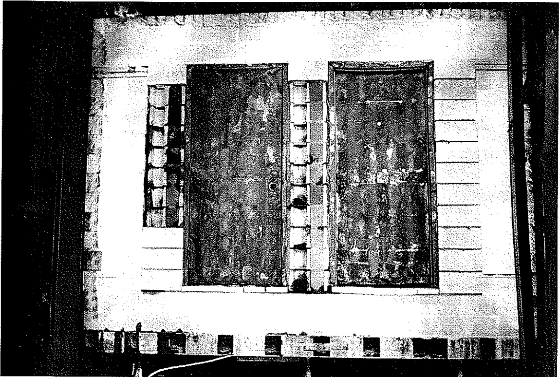
EXPOSED SIDE AFTER HOSE STREAM TEST
