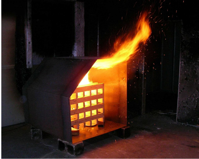
Figure 20. A simulated passenger compartment fire generated in a test
