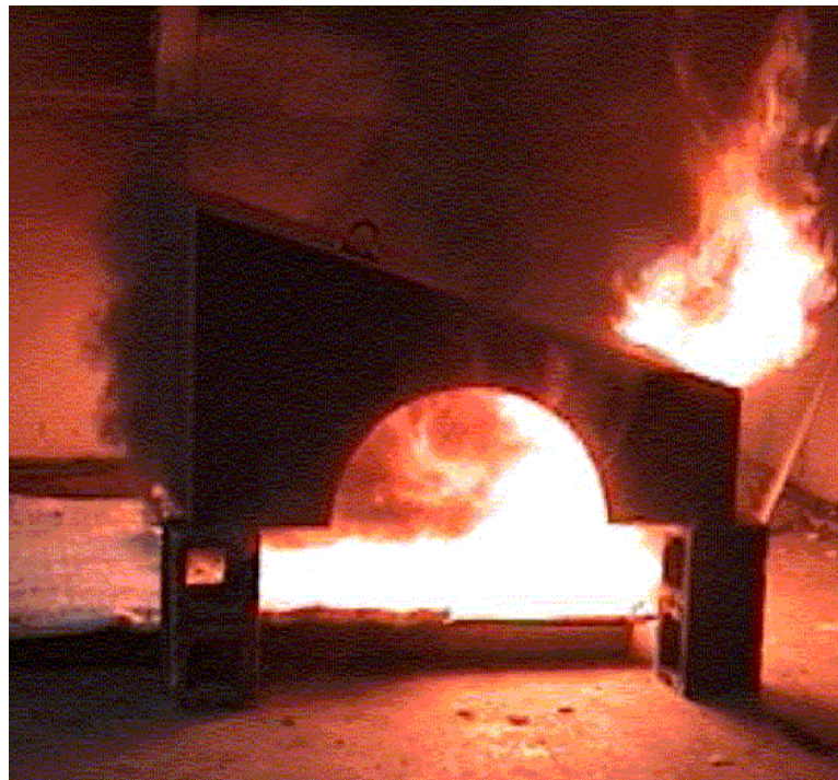
Figure 17. A simulated engine compartment fire generated in a test
