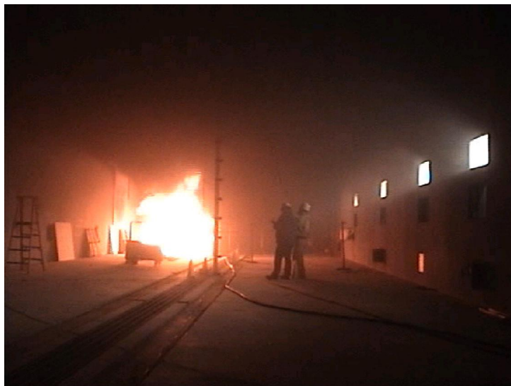
b). A simulated engine compartment fire at its full development stage in Test T-5
