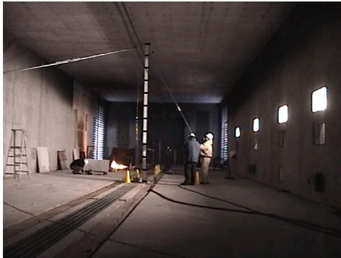
a). A simulated engine compartment fire at its initial stage in Test T-5
