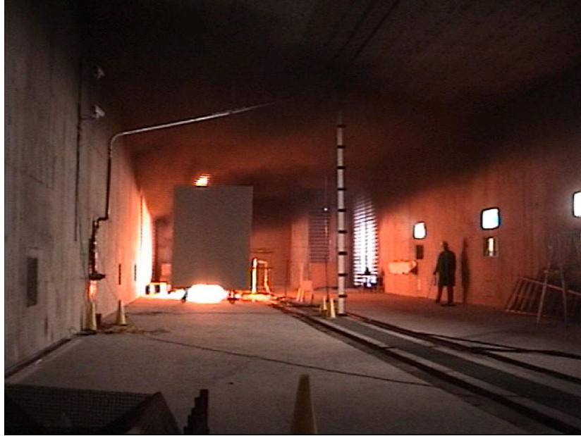
a). A 2.0 m 2 gasoline pool fire behind a large vehicle at 10 s after ignition
