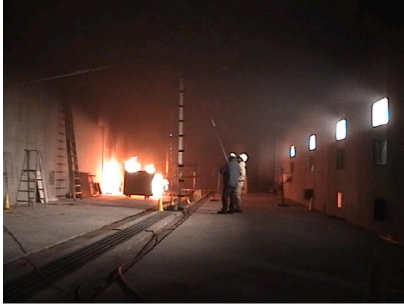
Figure 6.4. Tunnel conditions with a gasoline pool fire (1.0 m x 1.0 m) located underneath the simulated vehicle in Test T-7
