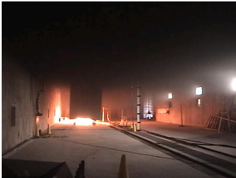
b). A 2.0 m 2 gasoline pool fire behind a large vehicle at 25 s after ignition
