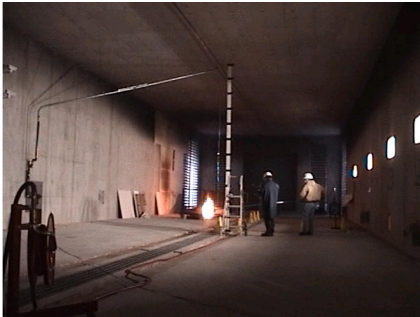
Figure 6.1. An open space gasoline pool fire in the test tunnel
