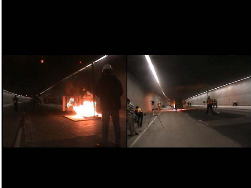
Figure 7.18. Photographs of a pool fire located behind a simulated vehicle taken from front and back of the fire setup with the fire was located at 32 m from the detectors
