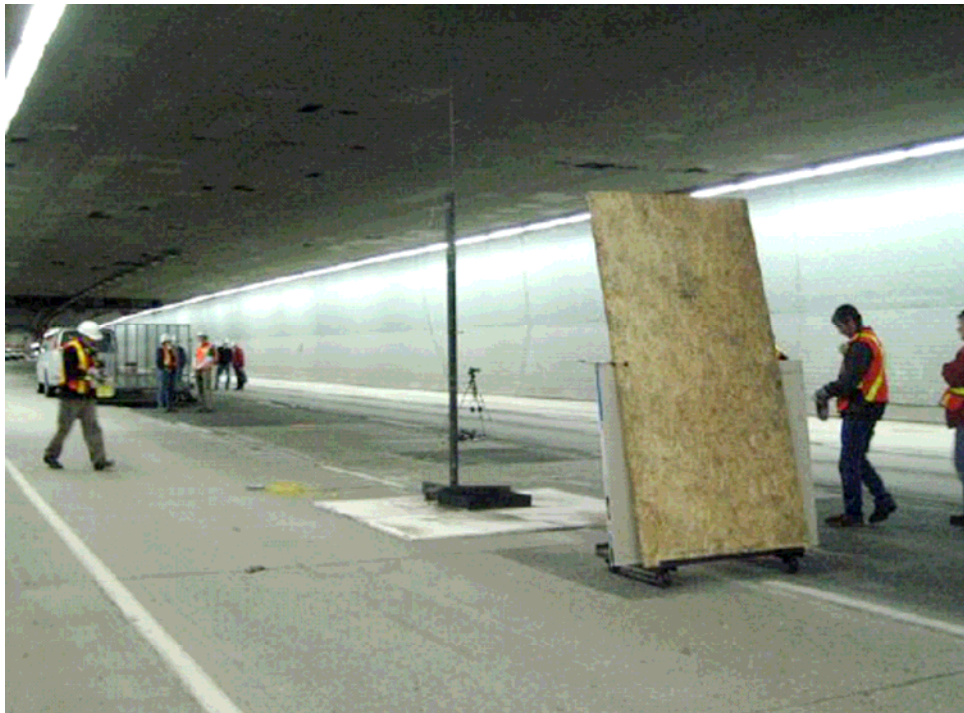
Figure 7.16. Photograph of the setup of a pool fire located behind a simulated vehicle
