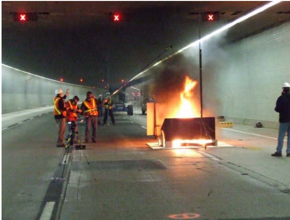
Figure 6.2. Measurement of air velocity at fire location during test
