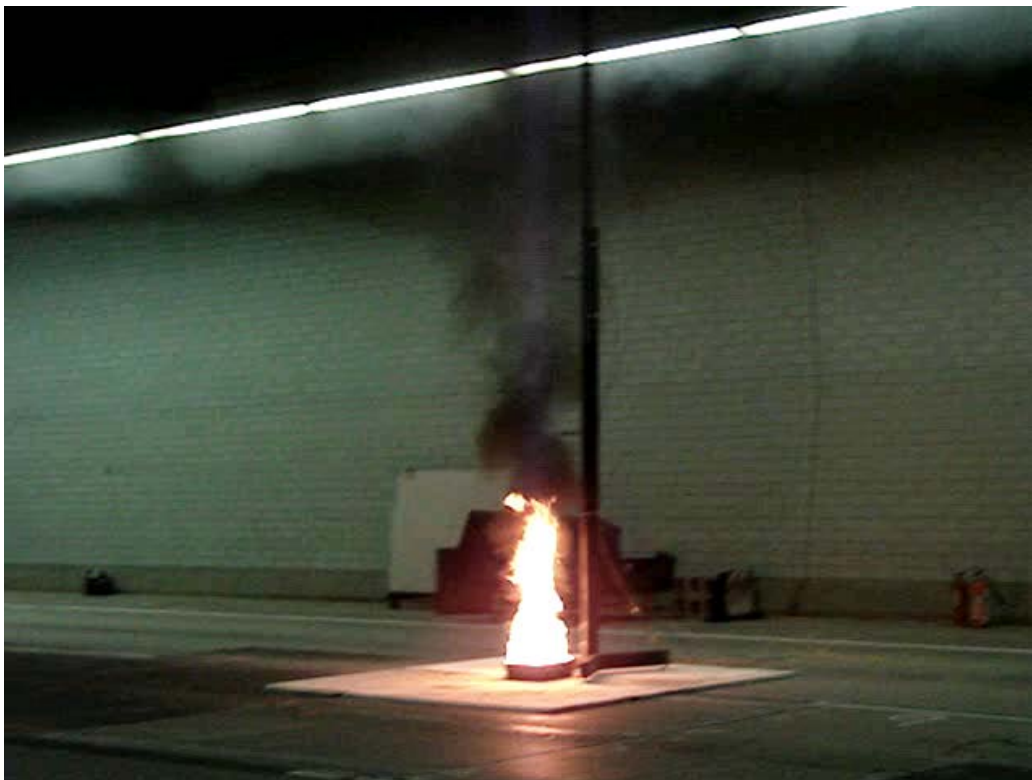
Figure 7.2. Photograph of a small open pool fire in Viger Tunnel tests
