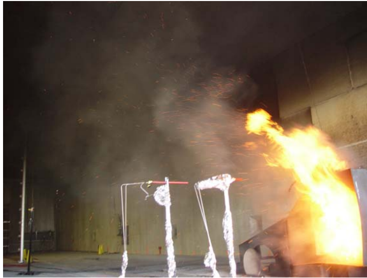
Figure 7.52. The side view of the simulated passenger compartment fire with wood cribs and foam with an airflow speed of 3 m/s
