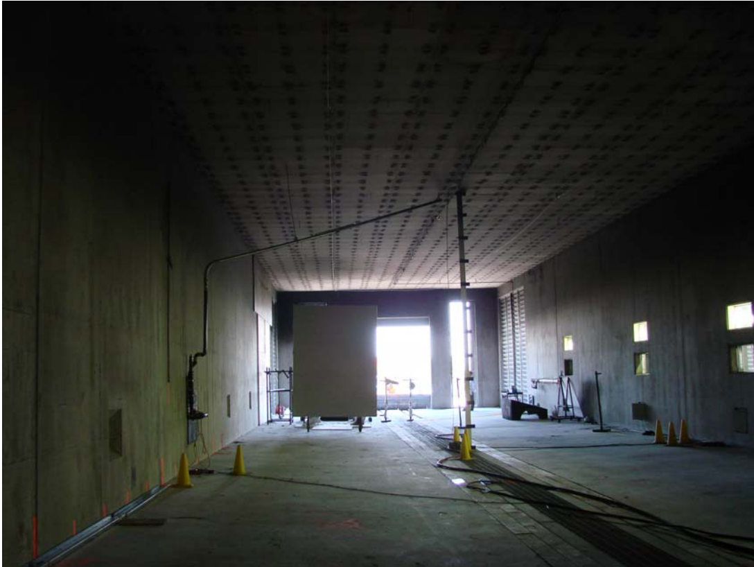
Figure 7.31. Photograph of the setup of a pool fire located behind a large simulated vehicle in the test tunnel
