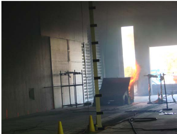
Figure 7.53. The front view of the simulated passenger compartment fire with wood cribs and foam with an airflow speed of 3 m/s
