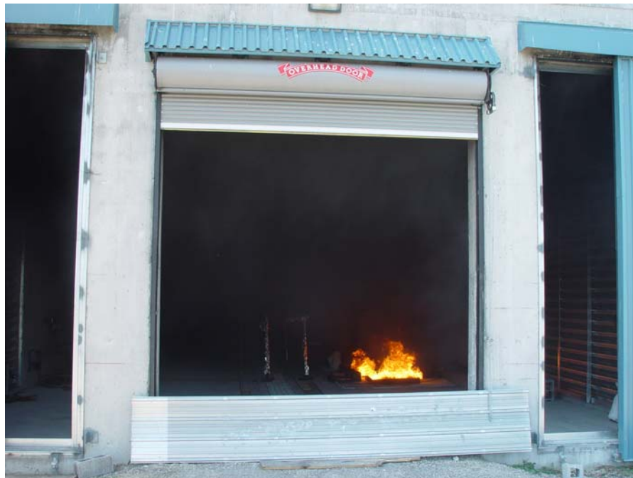
Figure 6.1. The setup of the door and the two side louvers at air velocity of 1.5 m/s
