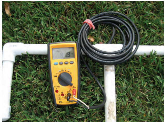
Meter connected to Test Rig probes
