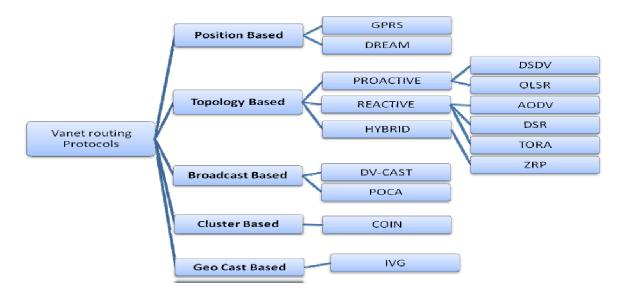
Figure 1: Routing Protocols in VANET
