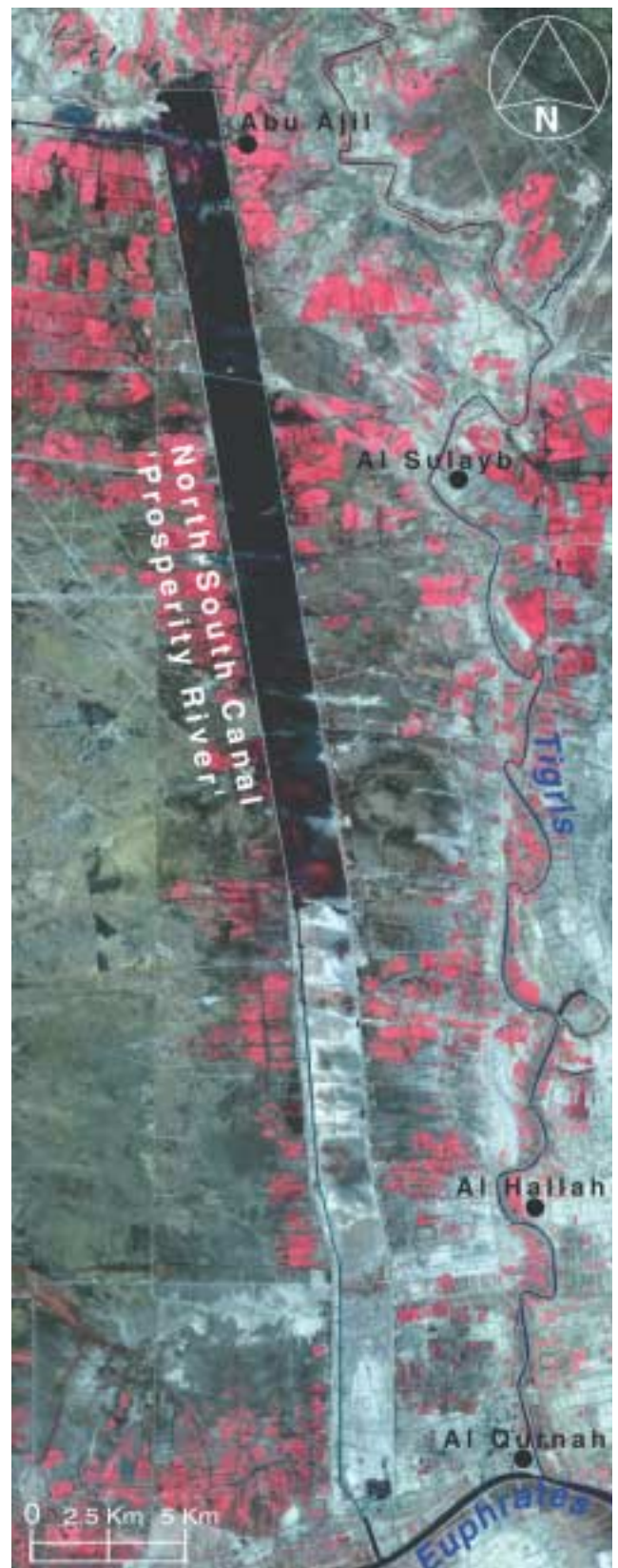
Fig. 19 - In 2000, the lower stem of the North-South Canal had largely dried-up leaving a narrow connecting canal to the Euphrates. (Landsat 7 false-colour image derived by merging of panchromatic ETM Band 8 with Bands 4, 3 and 2, taken on 26 March 2000).
