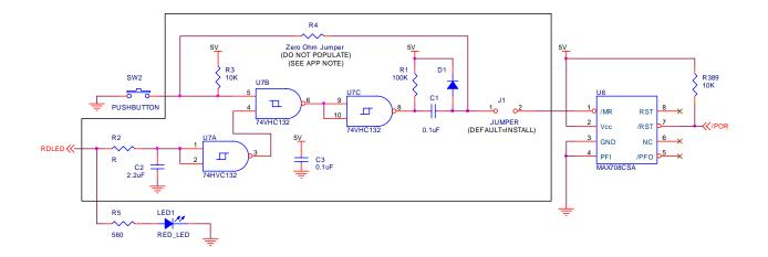
Figure 2. Proposed Reset Circuit 2
