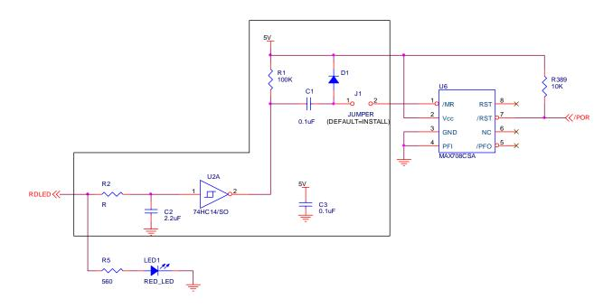
Figure 1. Proposed Reset Circuit 1
