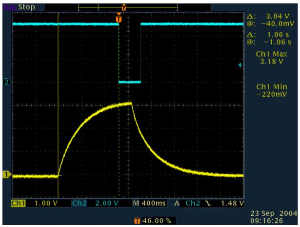
Figure 3. Oscilloscope View of the Red LED RC Circuit, R2 = 120 k $\Omega$
