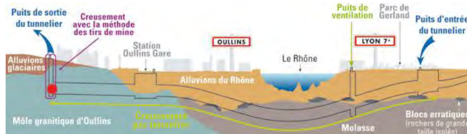
Figure 4-12. TBM arrival to the exit shaft
