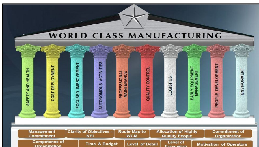
Figure 2: WCM pillars. Note that WCM is composed of ten major dimensions. Source: (FIAT, 2012).
