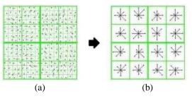
Fig. 2 A sample SIFT descriptor computation. (a) The gradients of an image patch around a keypoint. These gradients are then accumulated over  $4 \times 4$  sub-regions, as shown on the (b).The length of the arrow corresponds to the sum of the gradient magnitudes in that direction.
