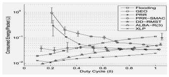
Fig. 4. Average energy consumption per packet versus duty cycle for different values of  $\Sigma$ Th.
