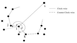
Fig. 2. Illustration of angle-based routing.
