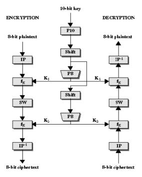
The 10-bit key is first subjected to a permutation (P10) and then a shift operation is performed. The output of the shift operation then passes through a permutation function that produces a 8-bit output (P8) for the first sub key (K1).
