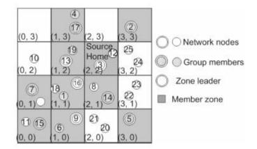
Fig. 5 Zone Based Structure for RSGM [11]
