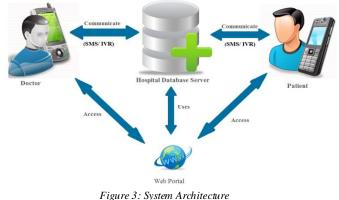
Hospital server automatically attends the call from patient and doctor through voice modem and resolves their queries. GSM modem is connected to hospital server that allows the server to receive the text message. Server automatically analyse message through text recognition technique. We are providing Web Portal another option of interaction with system. So by using the web portal patient and doctor can schedule their Appointments, also patients and doctors can view patient's diagnosis reports.
