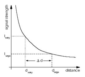
Figure: Signal Levels for Handover
