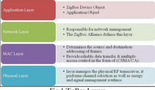
Fig.1 ZigBee Layers
