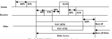
Fig.5 RTS/CTS Access Mechanism
