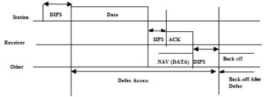
Fig.4 Basic Access Mechanism
