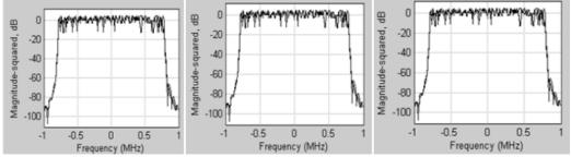
Fig.4 Frequency Spectrum of (a) Rician Channel, (b) Rayleigh Channel (c) AWGN Channel at 20 dB SNR
