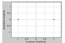
Fig. 2 Constellation diagram of BPSK transmitted signal
