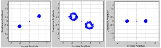
Fig.3 Received signal of (a) Rician Channel, (b) Rayleigh Channel (c) AWGN Channel at 20 dB SNR
