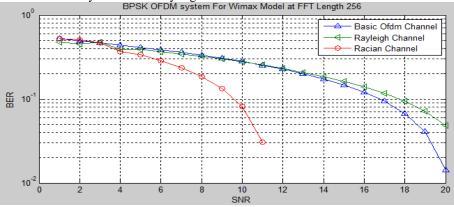
Fig. 5 BER versus SNR graph through AWGN and fading channels
