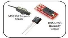
Fig. 3 Sensors Connected to Microcontroller Board
