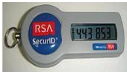
Figure 2: Hardware based product SecurID with a token
