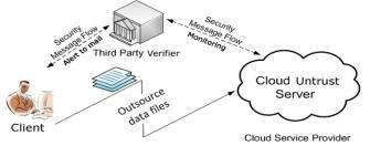
Fig. 2: The architecture of cloud data storage service with TPV
