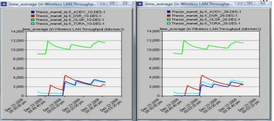
Fig. 3 Throughput - 5 sources at 10m/s and 28m/s
