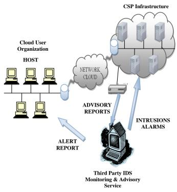
Fig 1 Architecture of Distributed multi tier IDS
