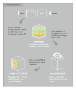
Figure 4 OpenStack Architecture
