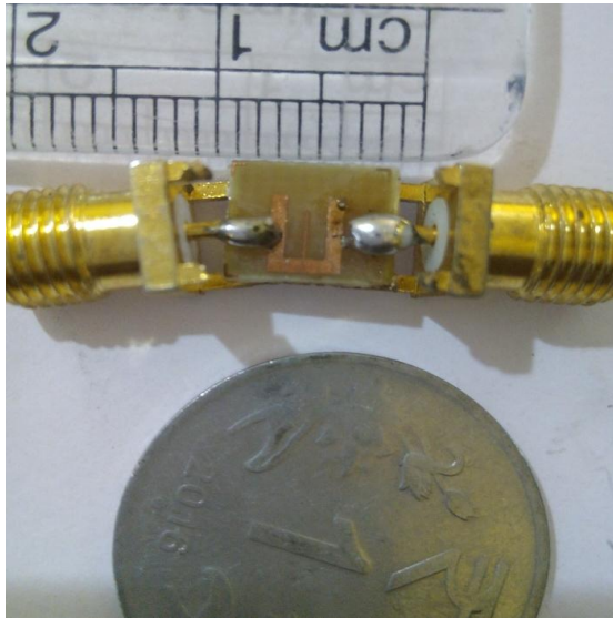
Fig.4. Fabricated Prototype of Proposed Primary UWB Filter Design
