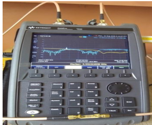
(b) Measurement Setup for Proposed Band Notched UWB Filter
