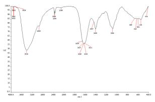
Figure 1 FTIR spectra recorded from powder of silver nanoparticles
