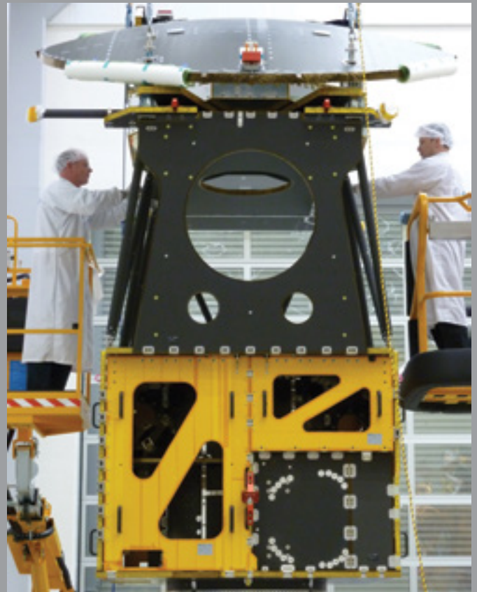
Integration fit-check of the Cloud Profiling Radar Structural Model on the EarthCARE Protoflight Model (Astrium/JAXA)
