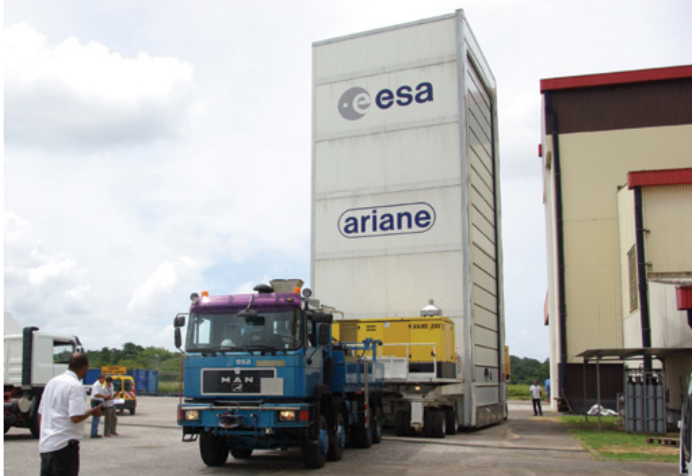
↑ When moving between the different buildings and launch sites at Kourou, strict thermal, humidity and clean conditions must be maintained during the moves. Here, the CCU-3 (Container Charge Utile) is a cleanroom on wheels
