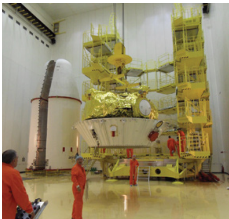
↑ The scaffolding used to prepare the upper composite. A Fregat upper stage, attached to a section of the launcher, is inside the scaffolding. The halves of the fairing are shown on the left
