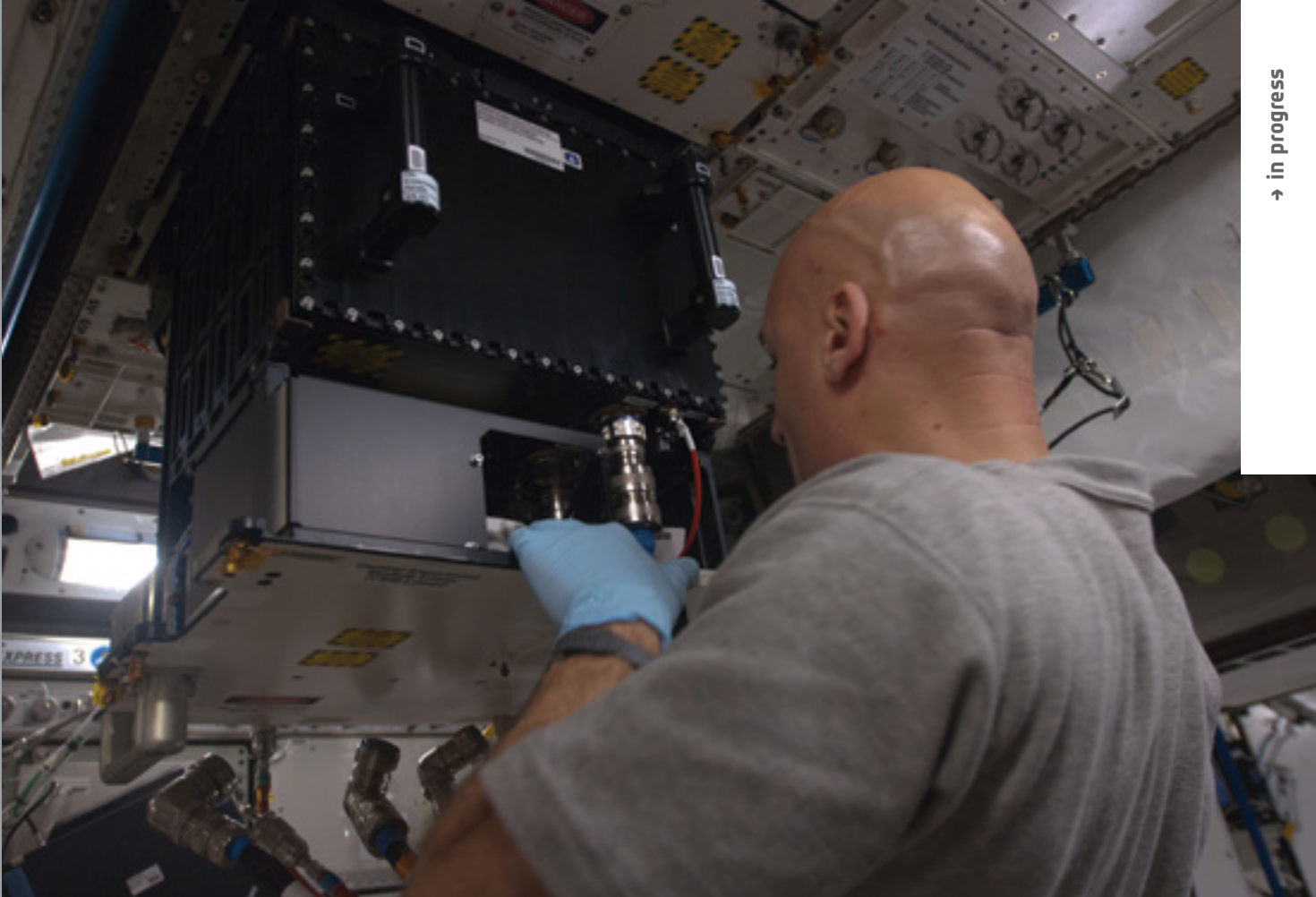
Luca Parmitano installs the Fundamental and Applied Studies of Emulsion Stability (FASES) experiment container into the Fluid Science Laboratory in Columbus
