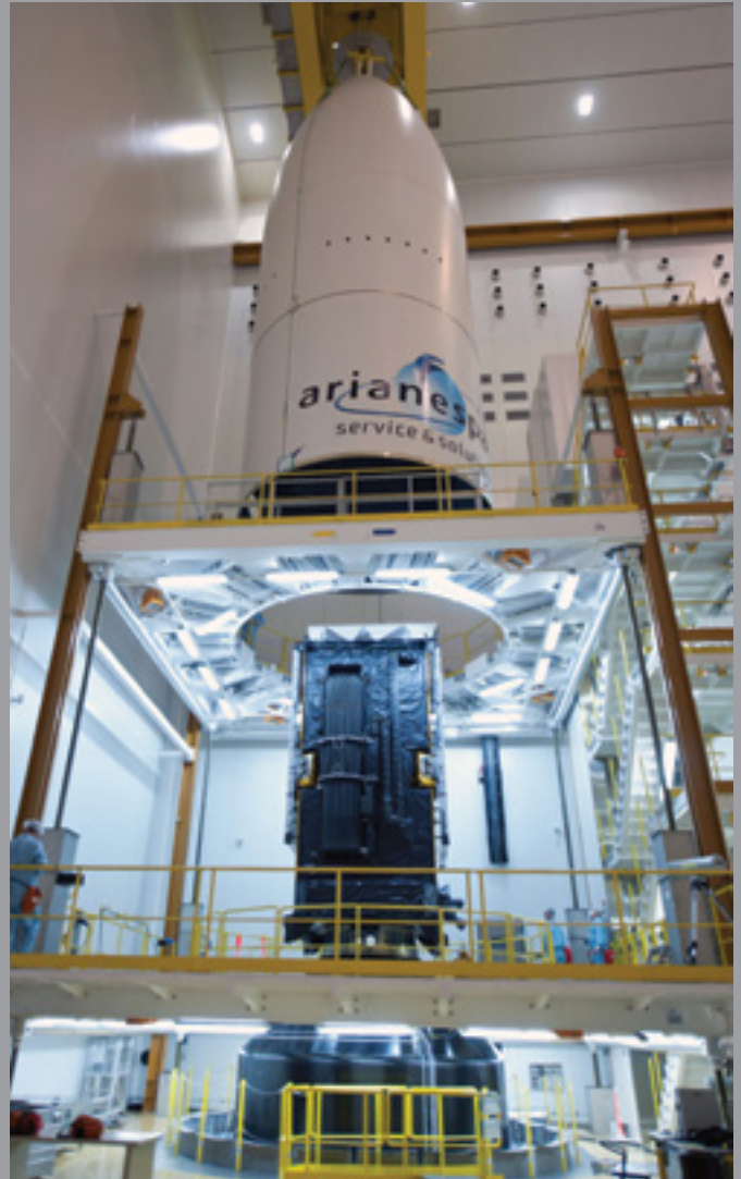
The last time Alphasat is seen before launch, as the Ariane 5 fairing is lowered to encase the satellite and the Sylda dual-launch pod (ESA/CNES/Arianespace/Optique Photo Video du CSG)
