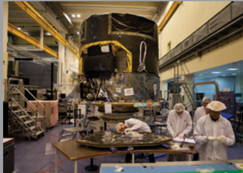
Final touches made to the Gaia solar panels in the Toulouse clean room (Astrium SAS)
