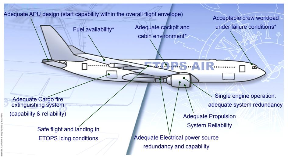
\* = Analysis considers failure conditions for the maximum diversion time/distance Relevant system safety assessments must take into account the maximum diversion time/distance
