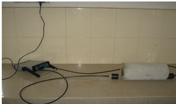
Fig.3.Ultrasonic Pulse Velocity test
