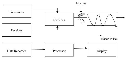
Figure 4.1 Basic block diagram of typical radar system
