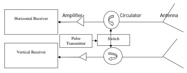
Figure 4.4 CV-990 polarimetric SAR system
