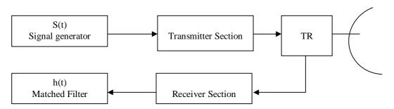
Figure 4.1.1 Matched FilterRadar System
