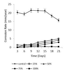
Figure 2: Variation in corrosion rate for mild steel in various concentrations of rosemary extract with passage of time.
