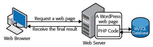
Fig3: Working relation of client, server and database in webCMS [6]
