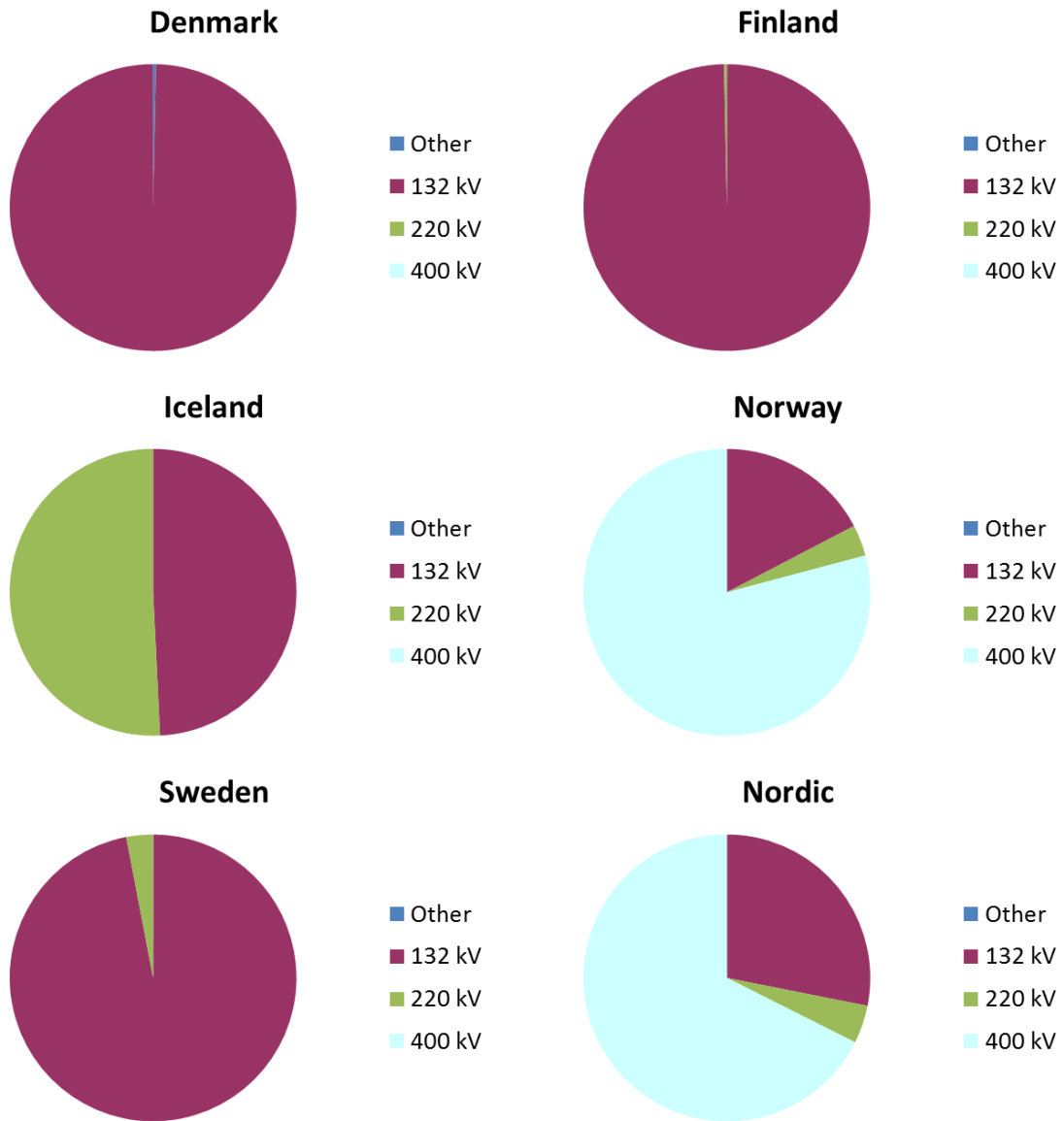
FIGURE 4.1.1 ENERGY NOT SUPPLIED (ENS) IN TERMS OF THE VOLTAGE LEVEL OF THE INITIATING FAULT IN 2013
